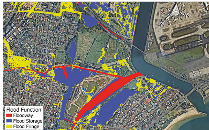
Figure 28 - Flood function mapping within Lower Muddy Creek
